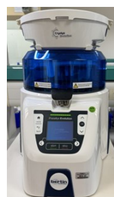
Left–Precellys® Evolution Homogeniser with Cryolys® Evolution cooling unit. Right–Plasma quenched with solvent
